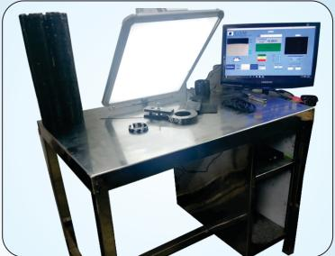
**ICAMCV100R** is a newly crafted machine vision system from NAACS with the aim of precise specific inspection in a cost effective manner in the field of Piston Ring manufacturing. Herein, we use a camera that measures the closed gap of each piston ring (Least count up to 4 microns) with the help of our intricately developed software.
