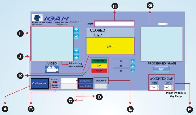
A This tab is used to calibrate the camera as per the actual gap size at the time of initiating a new batch. The first ring of the batch is placed in the ring gauge.
